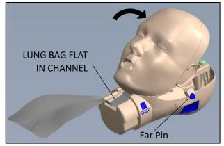
3.) Attach Face assembly onto Head Back by aligning first at chin and rocking back to engage ear pins. Confirm ear pins are fully engaged and Lung Bag is flat in neck channel.
